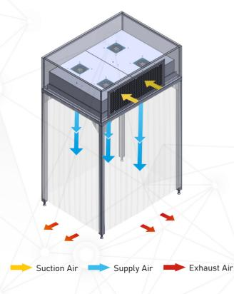
After passing through the HEPA filter, the clean air flows through a perforated stainless steel air distributor. This design ensures uniform distribution of laminar airflow across the entire working space, creating an environment with minimal turbulence and consistent air quality.
